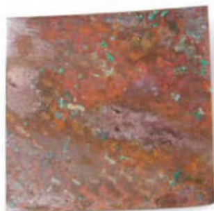
Immersed/Wrapped, Cotton, Vinegar+Salt: Copper
